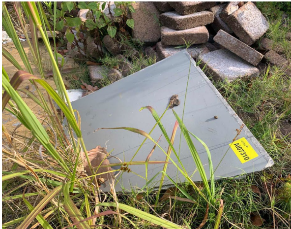
Line ID 31: External, The Compound, Throughout, South of Concrete Stockpile, Debris, Compressed Cement Sheet - No Asbestos Detected
